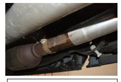
**3.** Install the hangers into the rubber grommets.
