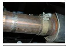
2. Install over axle pipe Item # A onto your factory head pipe using your factory clamp.Do not tighten.
