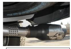
7. With proper clearance from spare tire install the exhaust tip onto the tailpipe. The system was designed to have the tip 1" below the quarter panel of the vehicle. With the tip in your desired position begin to tighten down all clamp connections from the front head pipe back
