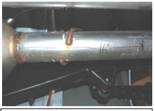
2. Short Beds: Measure 16" from the end of the factory Particulate Filter towards the axle .Mark 16" and use a hack saw or sawzaw for cutting.
