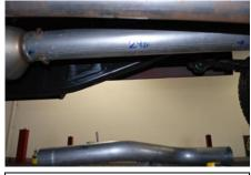
3. Long Beds: Measure 29" from the end of the factory Particulate Filter towards the axle .Mark 29" and use a hack saw or sawzaw for cutting.
