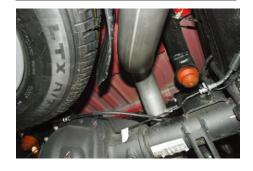
5. Install the exit pipe Item #B Be sure there is clearance from the spare tire and shock. You may need to adjust the pipes for a proper 1.50" of clearance.
