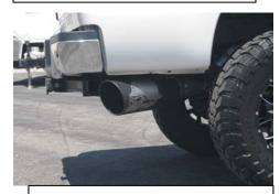
7. With proper clearance from spare tire and the tip in your desired position begin to tighten down all clamp connections from the front head pipe back to the tip.
