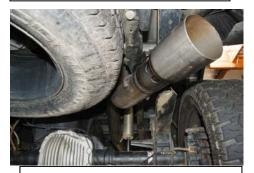
**5.** Install the exit pipe Item #C Be sure there is clearance from the spare tire and shock. You may need to adjust the pipes for a proper 1.50" of clearance.
