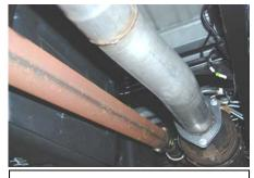
**3.** Install Head pipe Item #A onto the factory flange. Do not tighten until install is complete.
