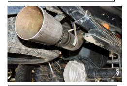
6. Install The Exhaust tip. The kit was designed to have a 1" clearance from the bottom of the quarter panel.
