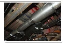
4.Use a jack stand to support the muffler assembly until you have installed the over axle pipe Item # C
