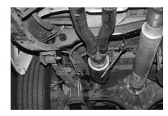
3. Install muffler assembly Item # D onto the Gibson head pipes. Slide the rubber grommet onto the welded hanger.
