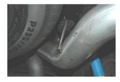
6. With proper clearance from the spare tire install the exhaust tip onto the tailpipe. The system was designed to have the tip 1" below the quarter panel of the vehicle. With the tip in your desired position begin to tighten down all clamp connections from the front head pipe back.
