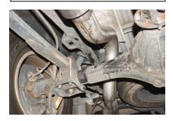
5. Install the Overaxle pipe Item # E into the muffler outlet. Install the rubber grommet and adjust system to properly fit your vehicle.
