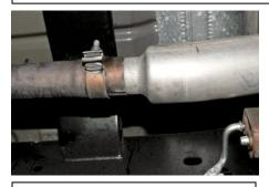
2. Install muffler assembly Item # A into the factory head pipe. You will re use the factory clamp at this connection. Install hanger into rubber grommet and loosely tighten down the clamp.
