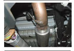
5. Install the over axle pipe Item # C into the muffler outlet. Install hangers into the rubber grommets. You may need to adjust the pipes to allow for proper fitment and clearance. Sometimes these adjustments will be needed at the front head pipes.
