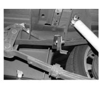
INSTALL HANGER # G ON THE PASSENGER TAILPIPE AND HANGER # H ON DRIVERSIDE TAILPIPE. MEASURE 19" FROM REAR OF FRAME AND BOLT INTO THE EXISTING ROUND HOLES (ABOUT 7/8") LOCATED ON THE FRAME ON BOTH SIDES OF THE VEHICLE.
