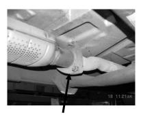
UNBOLT STOCK HEADPIPE AT THE 3 BOLT FLANGE DIRECTLY BEHINDTHE CATALYTIC CONVERTER. CUT STOCK TAILPIPE OFF RIGHT BEHIND THE STOCK MUFFLER. LEAVE ALL FACTORY RUBBER GROMMETS IN PLACE. SPRAY WD-40 ON ALL RUBBER GROMMETS FOR EASY REMOVAL.
