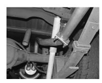
INSTALL PASSENGER SIDE TAILPIPE # C INTO THE MUFFLER 1-1/2" TO 2". ATTACH IT TO THE MUFFLER USING CLAMP #I. USE CLAMP # I TO HOLD TAILPIPE TO HANGER # F. DO NOT TIGHTEN
