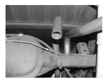
INSTALL DRIVERS SIDE FRONT TAILPIPE # D INTO MUFFLER 1-1/2" TO 2". USE CLAMP # J AND ATTACH IT TO THE MUFFLER. DO NOT TIGHTEN.
