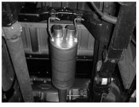
INSTALL MUFFLER #B ONTO HEADPIPE 1-1/2" TO 2" USING CLAMP #I + #k. INSERT WELDED HANGERS INTO RUBBER GROMMET. MAKE SURE OUTLETS ARE LEVEL. USE A JACKSTAND TO SUPPORT MUFFLER. DO NOT TIGHTEN.
