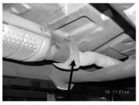
UNBOLT STOCK HEADPIPE AT THE 3 BOLT FLANGE DIRECTLY BEHIND THE CATALYTIC CONVERTER. CUT STOCK TAILPIPE OFF RIGHT
