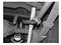
INSTALL PASSENGER SIDE TAILPIPE # C INTO THE MUFFLER 1-1/2" TO 2". ATTACH IT TO THE MUFFLER USING CLAMP # J USE CLAMP # J TO HOLD TAILPIPE TO HANGER # G. DO NOT TIGHTEN
