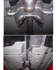
**2.** Install headpipe assembly #A onto stock Y-pipe. Secure pipe with clamp #C. DO NOT TIGHTEN. Use jackstand to support muffler.
