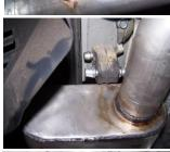
**4.** Insert all welded hangers into all rubber grommets.
