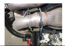
4. Next install the Gibson Muffler assembly. Install the top hanger mounts first then slide the inlet over the factory head pipe re using the factory gasket and springs. Once in position, install Headpipe and top muffler springs.
