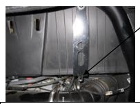
3. Next use a ¼" drill bit to drill the hole for the tailpipe brackets. You will drill the lower threaded hole on the both driver and passenger side rear bed bracket. See above photo for location. Drill hole on both sides of the vehicle.
