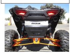
6. Install rear Gibson beauty plate. Use the factory bolts and supplied nylock nuts for the top two holes. Once they have been installed tighten the Gibson brackets at the rzr frame. Adjust plate for a level finish.
