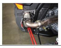
2. Once you have removed the heat shield remove the factory brackets and re install the Gibson supplied brackets #E using the factory bolts and factory location. Keep loose until final install.
