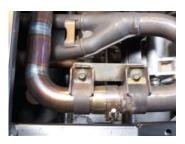
3. Now install Gibson mid-pipe onto stock header using supplied 1¾" band clamp. Then install stock band onto Gibson mid-pipe for extra support.
