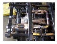
7. Now install the Gibson muffler and slide hanger rods into grommets. Then install the 3 supplied exhaust springs from the muffler to the midpipe.
