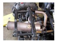
2. Remove stock band clamp off of factory muffler pipe. Now remove stock muffler assembly leaving the stock header attached.
