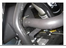
Install the headpipe into muffler make sure you slide the clamp onto the muffler first, use hardware provided to bolt down the headpipe. Next remove the exhaust gasket from the stock muffler and install into you new headpipe. (this is needed to seal the headpipe to header)
