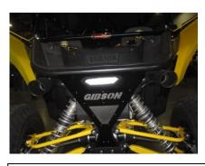
Adjust your kit so the tips are coming out level tighted all nuts, bolts and clamps. Re install rear shock by installing upper bolt first.
