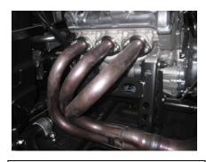
Re install your factory header using the stock hardware make sure to insert it into the new headpipe.
