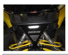
Adjust your kit so the tips are coming out level tighten all nuts, bolts and clamps. Re install rear shock by installing upper bolt first.
