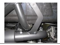
Next install tailpipe brackets onto exsiting bolt using the 6mm flange nuts provided use some red locktight on these leave loose till install is complete.
