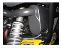
Install your Gibson muffler assembly into the frame using the hardware provided leave all hardware loose til the last step this is important for adjustments in the final step.
