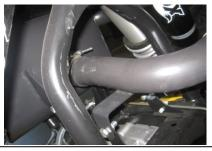
Install the headpipe into muffler make sure you slide the clamp onto the muffler first, use hardware provided to bolt down the headpipe. Next remove the exhaust gasket from the stock muffler and install into you new headpipe. (this is needed to seal the headpipe to header)
