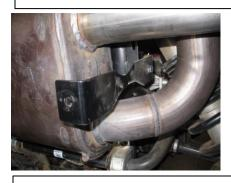
5. Install the provided heat shield bracket's into the factory locations re using the factory bolts to attach it to the frame on both driver and passenger sides.
