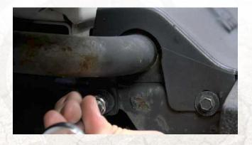
For OEM bumpers, using a T55 Torx, remove the four (4) top front bumper hardware and tow hooks (if
