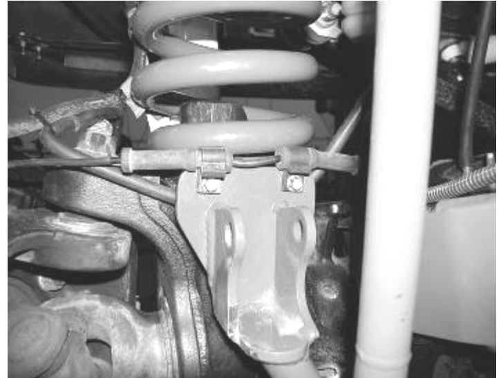
Picture shows coils already installed for proper ABS placement
