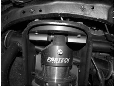
2.) Attach the bearing spacers to the lower rod end of the shock. Taller spacer should face the front of vehicle and the shorter spacer to the rear of the vehicle. 3.) Slide the lower rod end into the lower shock mounting plate of the control arm and install bolt.
