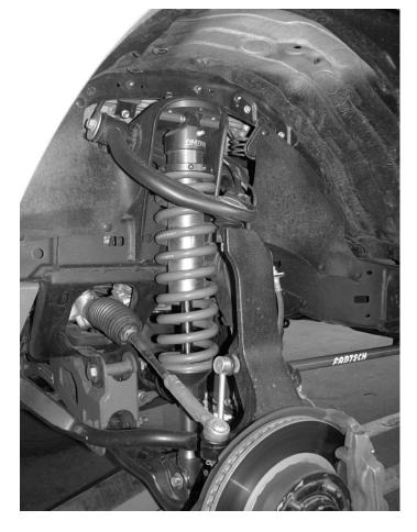
4.) Now move to the passenger side and repeat the procedures for the installation of the Coilover. Once both sides have the newly installed Coilover, reinstalled the sway bar links on both sides and also reinstalled the tie rod ends. You have now completed your installation. Spanner wrench is not included in this kit if needed order FTS98008. We recommend driving the vehicle for 50 miles and retorque nuts and bolts and then have it aligned to factory specs.
