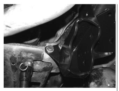
16. Locate and insert the three FT177 frame sleeves into the three holes in the side of the frame. Re-install the pocket using the supplied 1/2" hardware. The rear bolt uses a flat washer on the bolt on both sides of the frame and nut tab FT44154. The front of the pocket gets the 1/2" button head bolt with one flat washer and nut tab FT44152. Torque the 1/2" hardware to \*\*127 ft-lbs and the 14mm hardware to \*\*215 ft-lbs. SEE PHOTOS BELOW.
