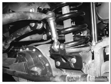
32. Working with both sides, locate FT44137 Brake Line Bracket & the supplied 1/2" x 1-1/4" hardware. Drill the factory mount on the axle and the brake line bracket to 1/2". Attach the Fabtech bracket to the factory mount on the axle with the 1/2" bolts. Attach the brake line bracket to the new Fabtech bracket. Torque to \*\*127 ft-lbs. SEE PHOTOS BELOW.
