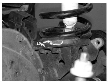
23. Connect the track bar to the new drop bracket using the supplied 9/16" x 3" bolt, nut and washers SEE PHOTO BELOW.
