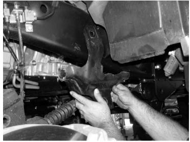
14. Support the transmission crossmember and remove the two bolts that secure the crossmember to the frame. Discard the hardware. SEE PHOTO BELOW.
