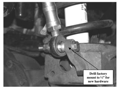
19. Locate the supplied ½" button head bolts and the sway bar bushing along with the cup washers. Attach the bushing end of the sway bar end links to the sway bar, leave loose at this time. At times this may be easier to attach when the truck is completed and on the ground. SEE PHOTO ON NEXT PAGE
