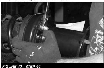
43. Install the coil over into the frame bucket. Rotate lower mount inline with the control arm tabs, and the pivot at the control arm using the factory hardware. Torque the upper nuts to 35 ft-lbs and the lower pivot to 100 ft-lbs.
