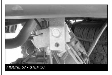
59. Locate and install the rear lift blocks FTBK52. The extended bump stop perch will be facing inboard of the truck. Using the provided u-bolts, nuts and washers, align the axle, lift blocks, and springs and torque u-bolts to 90 ft-lbs. SEE FIGURE 58
