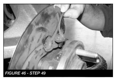
50. Carefully pull some slack from the frame side and reconnect the vacuum line to the hub assembly. Install the Fabtech frame brake line bracket (FT70032). Using the factory hardware, mount factory brake line bracket to the side of the Fabtech knuckle. After installing the factory brake line bracket, check to insure full movement by steering the knuckle back and forth, and make sure none of the ABS lines, brake lines, or vacuum lines are inhibited during full test movement of the knuckle.
