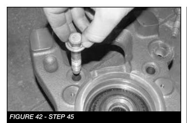
46. Locate the factory 4WD actuator and install into the Fabtech spindle. Torque the factory 8mm bolts to
