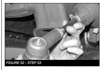
54. Reconnect the tie rod end to the steering knuckle and torque to 60 ft-lbs. **SEE FIGURE 53**
