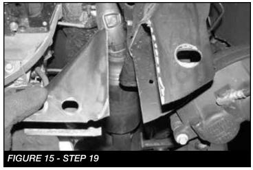
20. Still working on the driver side rear lower control arm pocket, locate the tab on the pocket closest to the front of the vehicle. You will need to sand a radius in the front side of the pocket in order to clear the differential housing. SEE FIGURE 16
