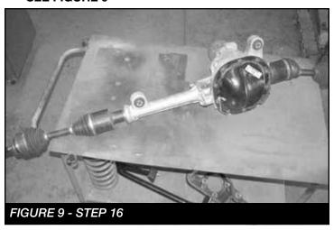
Locate rear differential mount closest to the pinion shaft.
