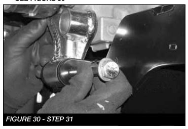
32. Support the diff to make sure the block on the diff is centered with the hole in the rear bracket.
