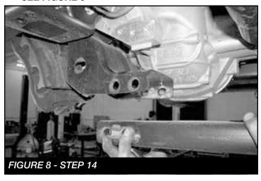
15. Remove the front drive shaft bolts where they attach to the front differential. Support the end of the driveshaft before removing the front differential.
