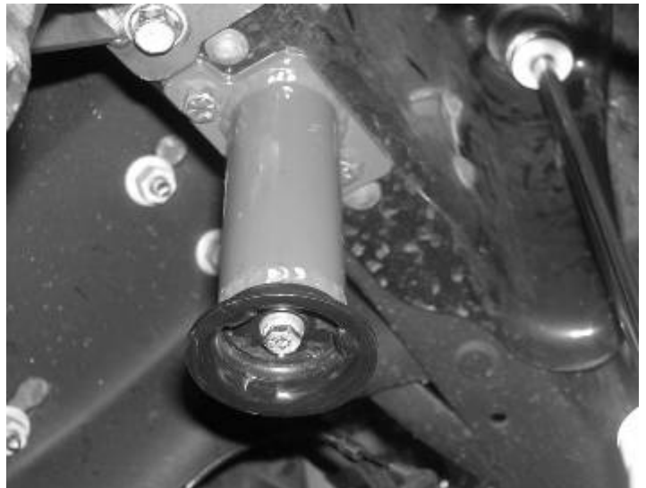
Photo shown without bump stop installed
