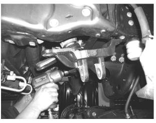
8. Remove the factory pitman arm from the steering box using a large pitman arm puller or large two-jaw puller. Save the hardware and discard the pitman arm. SEE PHOTO BELOW.
