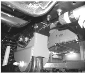
15. Reinstall the radius arm onto the truck using the original hardware. Attach to the axle first then to the new drop bracket using the reward hole. Leave loose at this time. SEE DRAWING IN NEXT COLUMN.
