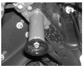
Photo shown without bump stop installed
