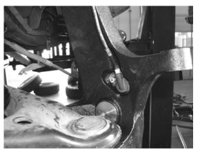
25. Route the ABS line from the sensor up the backside of the spindle. Using the supplied Adel Clap and 1/4" x 3/4" bolt and washer attach the line to the spindle. SEE PHOTO NEXT PAGE.
