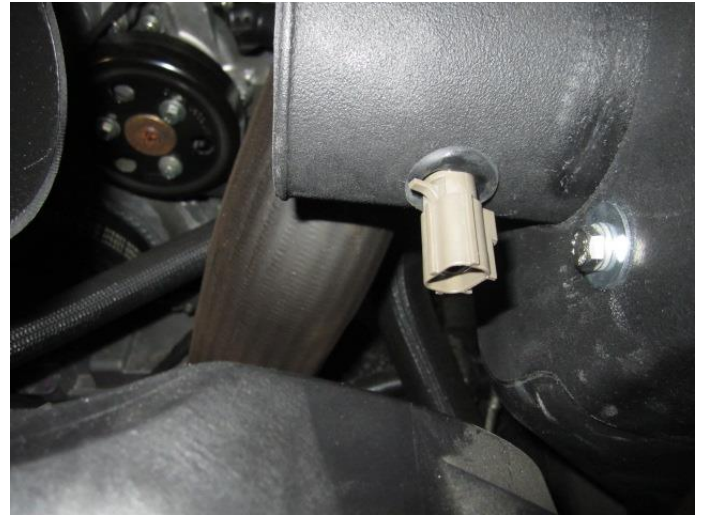
14. Press the ATS sensor into the rubber grommet on the CORSA filter adapter.
