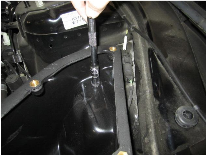
13. Tighten the air box in place using the factory 10mm bolt.
