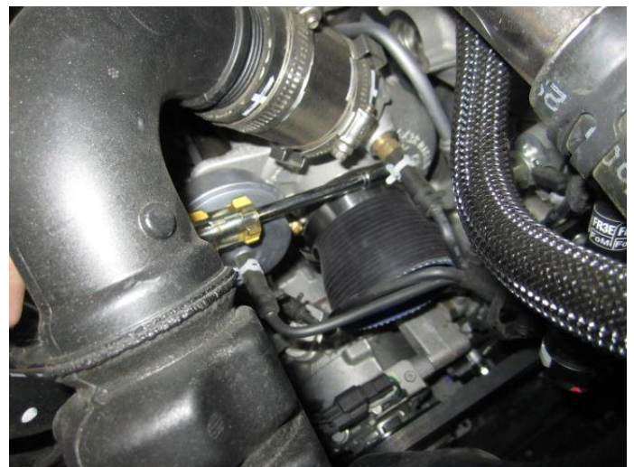
16. Attach the 2.5 to 3in reducer onto the turbo using the supplied #40 clamp using a 5/16 socket or nut driver only.
