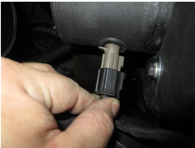
15. Attach the ATS sensor harness to the ATS sensor.
