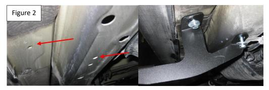
**Step 4:** Install rear bracket with provided hardware. Note you must enlarge outer hole to ½ inch in order to install provided M8 special nut.Install bracket as per Figure 3. Do not tighten.
