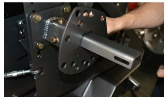
NOTE: Some tire/wheel combinations, such as 12.50 wide tires on stock Jeep wheels, may require more Overall Offset than the adjustment in the Tire Mount components allows (approximately 4-3/4" to 6-3/4"). In these cases, source a wheel spacer of suitable thickness to make up the difference.
