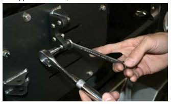
26. Install the V-Alignment Plate on to the back side of the Tire Carrier using the supplied hardware.
