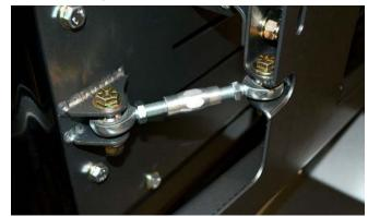
**29. Leave the jam nuts on** the turnbuckle loose, and adjust the length of the tie rod by rotating the turnbuckle. Adjust the length so that the V-Alginment Plate just begins to touch the V-Alignment Bushing when the tailgate is about 1/2" from being fully closed and latched. This is approximately the point at which the tailgate begins to compress the
