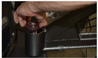
**21.** Apply some anti-sieze thread lubricant to the threads on the spindle. Install the large 1" Flat Washer next on the spindle, followed by the 1"-14 Lock Nut. Tighten the lock nut until it just touches the washer and bearing,
