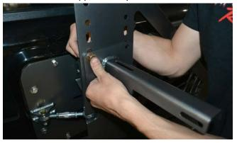
**32. Look at the Tire Mount** - Tire Side, and note that there are wheel stud holes for several different bolt patterns. Use the Bolt Pattern Template provided at the end of these instructions to determine which THREE holes to use for your specific bolt pattern. Once the three holes are correctly identified, mark them with a felt-tip marker.
