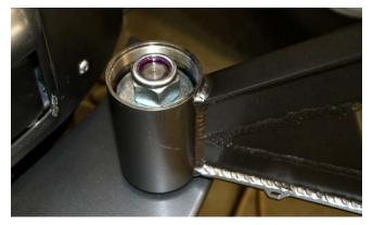
We can not supply a torque specification for this nut, just get it as tight as it takes to properly seat the bearings and provide smooth operation of the tire swing without any "play". Re-tighten this nut after the weight of the spare tire and accessories have been added, and again after a few days or a hundred miles of use. You may need to re-tighten this nut several more times until it permanently seats.
