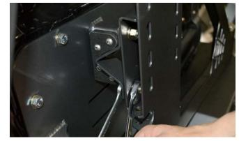
**28.** Assemble the Aluminum Turnbuckle, Spherical Rod Ends and SS Jam Nuts into a tie-rod assembly. Note that there are left hand threaded and right hand threaded ends of the turnbuckle, rod ends and nuts. (NOTE: the Turnbuckle Assembly may have already been preassembled at Poison Spyder). Use the provided hardware to attach one end of the tie rod to the Tailgate Plate, and the other end to the corresponding tabs in the back side of the Tire Carrier, as shown.
