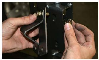
**27. Test that it seats correctly** into the V-Alignment Bushing on the Tailgate Plate when the Tire Carrier is closed against the tailgate. Adjust as necessary then tighten all fasteners.
