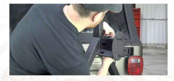
Install the 12mm bolt, with washers and nyloc nut, through the back of the tire carrier and brake light bar.
