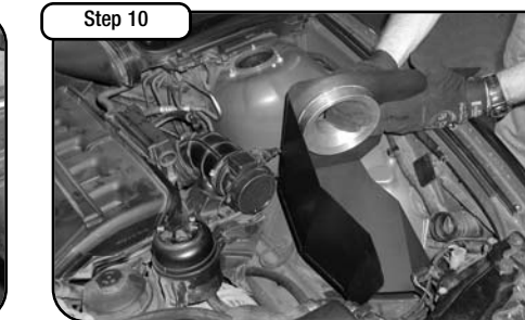
Install housing into vehicle, making sure to guide MAS into billet adapter.
