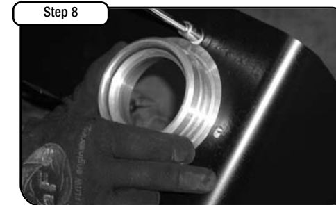
Install the billet aluminum adapter to the housing using M6 button heads supplied. Install factory o-ring into billet adapter.
