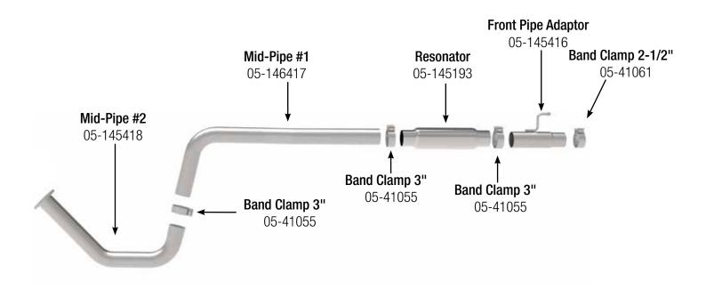
Professional installation is highly recommended. (Read instructions prior to installation). Make sure to always have at least (2) stands or jacks on hand to support the removal of OE system. Also for the installation of aFe system. Any Removal of rubber isolation mounts may require using a spray lubricant such as WD40 and a pry bar.
