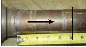
Step 7: Install the aFe race pipe using the OE V- band clamp, but do not tighten. Slide the adapter pipe over the aFe race pipe.
