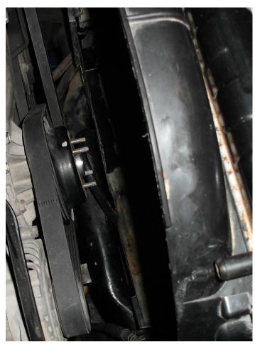
13. Remove the nuts securing the fan to the water pump.
