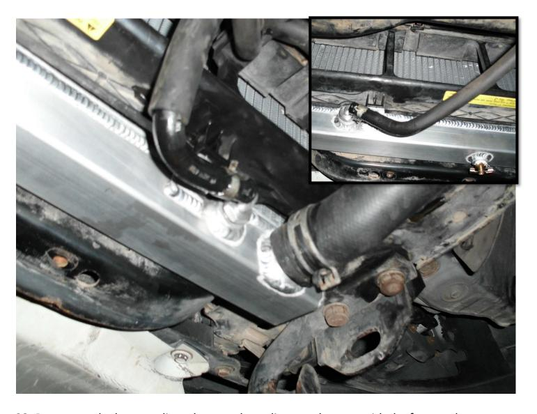
28. Reconnect the lower radiator hose to the radiator and secure with the factory clamp.
