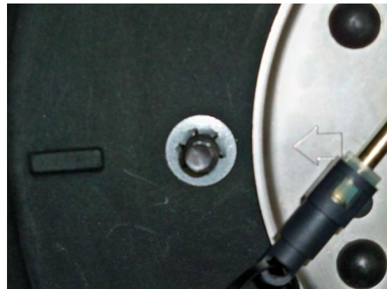
(Fig. 6) Line the arrow on the top of the PS-123 Sending Unit with the mark on the side of the sending unit mounting hole.
