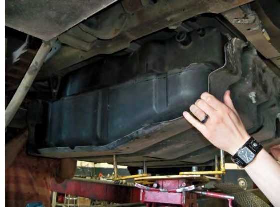
(Fig. 14) Lift tank into vehicle.
