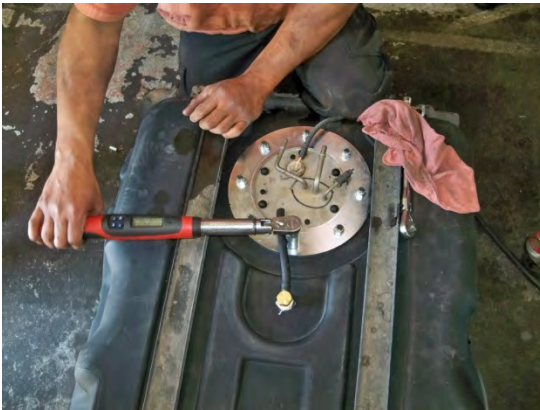
(Fig. 7) Using a torque wrench, tighten the flange nuts to 25 ft. lbs. using a "star" pattern. "Crash Flange" is not shown in this picture.
