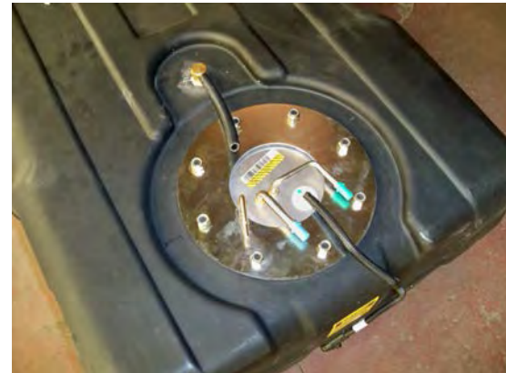
(Fig. 8) PS-123 Sending unit complete with "Crash Flange" installed in new TITAN tank.
