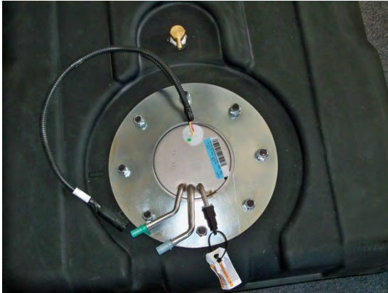
(Fig. 13) PS-191 Sending Unit Installed in TITAN tank.
