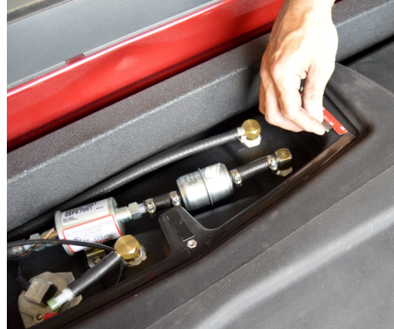
(Fig. 17) Showing completed plumbing and wiring on tank body. Tape backing is being removed in preparation for installation of the cover.
