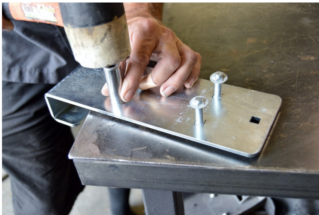
(Fig. 6) Use a deep socket to install Push Nut Retainer on 3/8" carriage bolts as shown.
