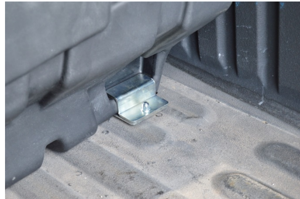
(Fig. 11) Toe clamps installed on Mounting Brackets
