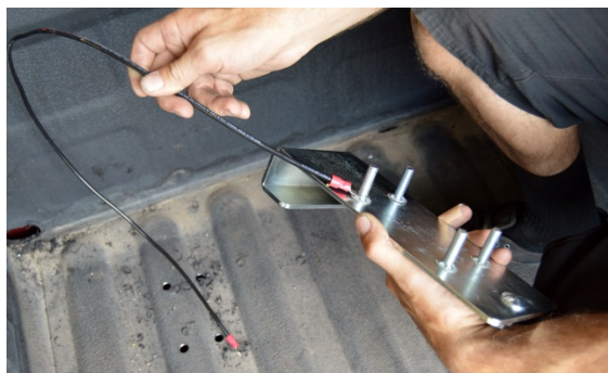
(Fig. 7) Install "99 0173 0000 Ground Wire Assembly" on front bolt in the "99 0000 0830 Mounting Bracket" which is to be installed on the driver's side of the vehicle.
