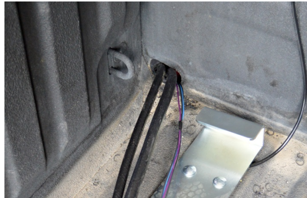
(Fig. 2) Fuel lines and wire loom can pass through plugged holes on vehicles so equipped.
