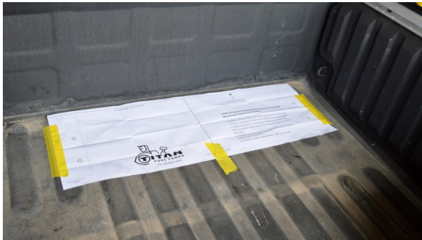
(Fig. 4) Template for drilling mounting holes taped down.
