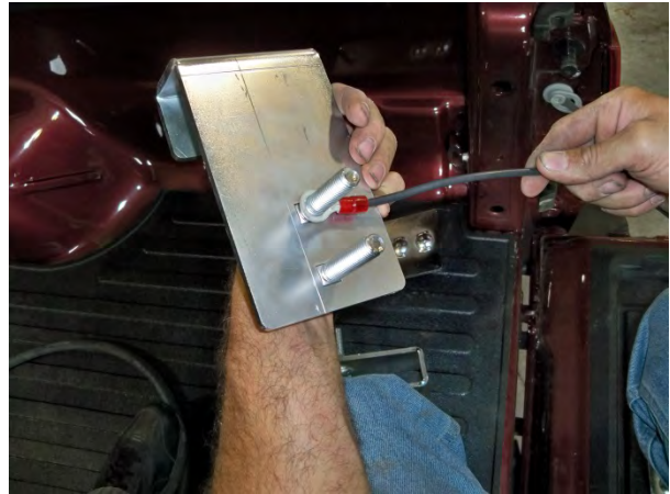
(Fig. 5) Install "99 0104 0000 Grounding Wire Assembly" on \frac{1}{2} " stud of the "99 0000 0129 Front Toe Clamp" to be installed on the driver's side of the vehicle.
