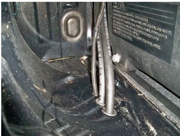
(Fig. 1) Holes for fuel lines and wire loom to pass, Model 5410060.
