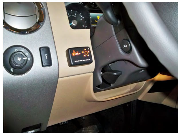
(Fig. 24) TITAN™ Electronic Controller mounted on dash.
