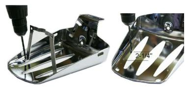
3. Drill U-bracket legs from  $^3/_{16}$ " holes to  $^{1}$ 4". Install supplied  $^{1}$ 4"-28 x  $^3/_{8}$ " Allen bolt and lock nut through one side of rack and bracket. Bend bracket to reach other side of rack, then install second Allen bolt. Install luggage rack to the backrest and U-bracket to the top of the license plate mount.
