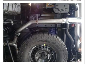
Step 4. Next loosely attach the Driver Side Tailpipe to the Y-Pipe by using the hanger brackets and the supplied 2.50" clamp.
