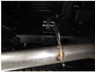
Step 6. Next loosley attach the Passenger Side Tailpipe to the Y-Pipe by using the hanger brackets and the supplied 2.50" clamp.
