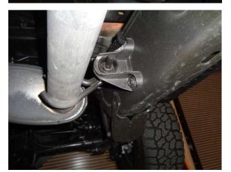
Step 1. To remove the OEM exhaust system, you will to need to remove the spare tire first. You can then disengage the welded hangers from the rubber insulators and remove the tailpipe assy. Unfasten the clamp attaching the OEM inlet pipe assembly to the catalytic converter. Do not damage or discard the inlet pipe clamp or rubber insulators as they will be re-used to mount the new system. Disengage the inlet pipe assembly hanger and remove the exhaust from the vehicle.
