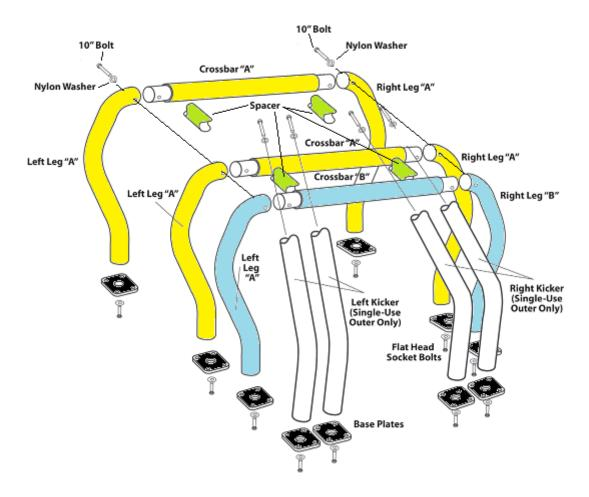
Refer to the installation instructions included with the Main Bars and Kickers for the assembly sequence.
