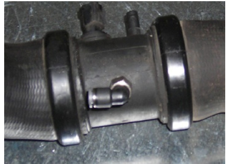
Nozzle & Nozzle Holder Mounted to Cold Pipe
