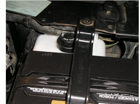
Tank Mounted Behind Battery
