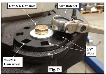
Step 28: Torque the previously installed 1/2" X 6 1/2" bolt to 80 ft./lbs. (Fig. P)
