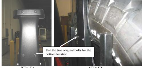
(Fig E) (Fig F) <u>Step 6:</u> Mount the tire stop bars on the outside holes on the tire carrier. The long end of the bars go toward the top. Mount each bar using the included 8x70mm bolts, flat washers and spacers and secure tightly. (Use two spacers for each bolt, they go between the
