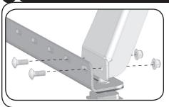
A. Uprights are paired. Mount an upright at rear left side (shown)and front left side (behind cab) to last pair of holes at each end of rack rail. Use 2 carriage bolts with serrated flanged nuts. Turn nuts fully tight now. Repeat procedure on passenger side.
