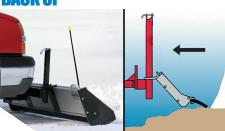
When backing up, the blade lies back. skimming over the ground. When driving blade automatically forward. re-engages for plowing. All you do is drive.
