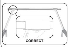
C. CORRECT. Cross bar centered without binding between uprights- bar is level and ready for next step.
