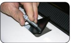
C. Maneuver corner of clamp into stake pocket by pushing down on foam and wiggling clamp until all 4 sides are inside of stake pocket.
