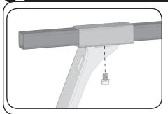
A. Start a Hex Head bolt ( $^3/_8$ " x  $^{1/_2}$ ") at each upright and turn it until serrated flange tightens up against upright.
