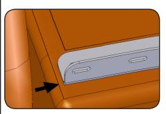
B. Align front of rail close to front edge of box-do not allow rail to go beyond front edge of box.
