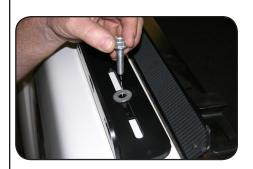
C. Place flat washer over slotted hole and turn a hex head bolt (3/8" x 11/2") on until finger tight. Ensure that alignment plate is aligned with stake pocket. Turn bolts in finger tight at remaining stake pockets.
