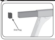
A. At each end of cross bar, tap end plug into tube.
