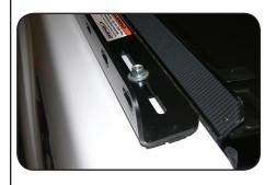
D. Slowly close tailgate to make sure it will not rub against rack rail when closed. (Adjust rack rail forward if needed). Now fully tighten all rack clamp bolts. Repeat steps 1 and 2 for rack rail on opposite side of box.
