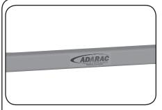
A. Repeat Step 4 shim placement and insert rear cross bar with reflective logo facing out towards rear. Repeat Steps 5 and 6 to finish mounting rear cross bar.
