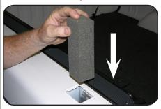
NOTE: Stake pockets must be open to install this product. Remove any accessories or snap-in stake covers if present.
