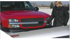
To begin plowing, remove pin, lift blade one end at a time and lower it over push frame, then replace the pin.
