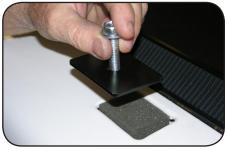
B. Orientate stake pocket clamp plate with smooth side up and thread a bolt  $(\frac{3}{8}$ " x  $1^{1/2}$ ") on several turns as shown.
