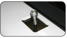
D. Adjust assembly until bolt is centered in stake pocket and clamp is fully supported by foam block. Carefully turn bolt out, allowing foam to support clamp for remaining steps.
