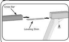
A. At each front upright slide leveling shim inside tube opening and hold them there while sliding cross bar (without ADARAC reflective logo) through each upright. Center bar on both uprights. Align shim hole with bolt hole in upright.
