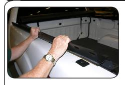
A. Carefully place rack rail (with warning decal) on top of box driver side. Adjust its slotted holes in line with holes on clamping hardware inside stake pockets.
