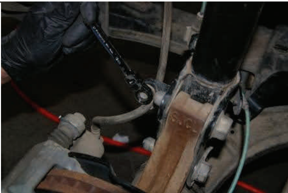
Reattach brake line bracket
