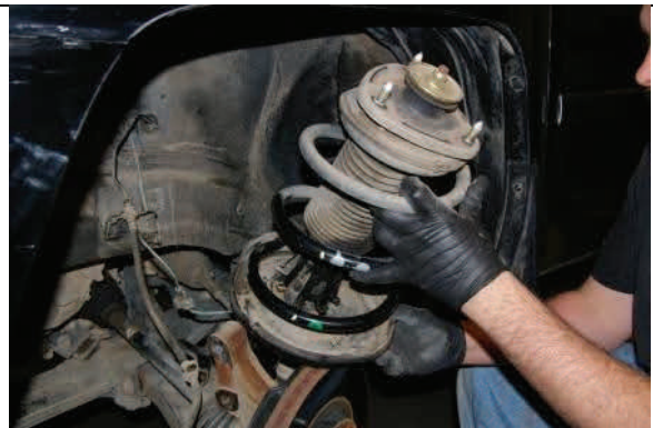
Lower suspension and remove strut. Caution: CV boot
