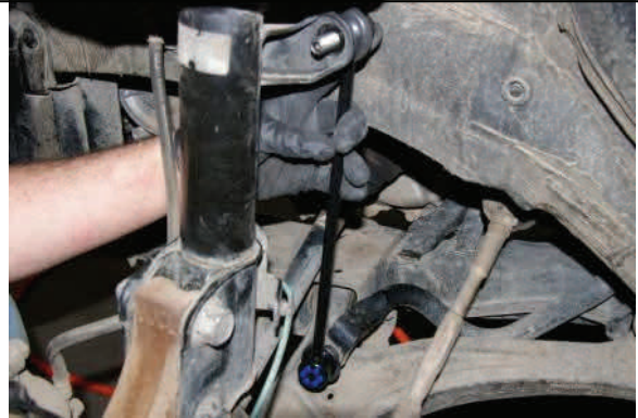
Raise jack attach top strut mount and new sway bar endlink
