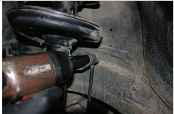
Disconnect and remove front sway bar end links
