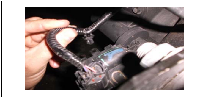
6. Unhook the wheel speed sensor wire line from the mount on the passengers side.
