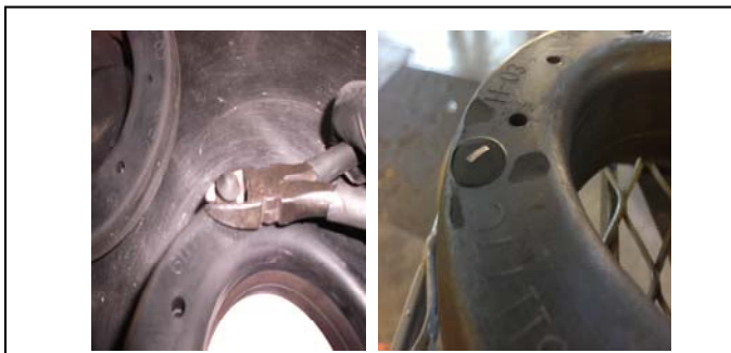
12. On OE spring isolator, cut off the rubber locating tab.
