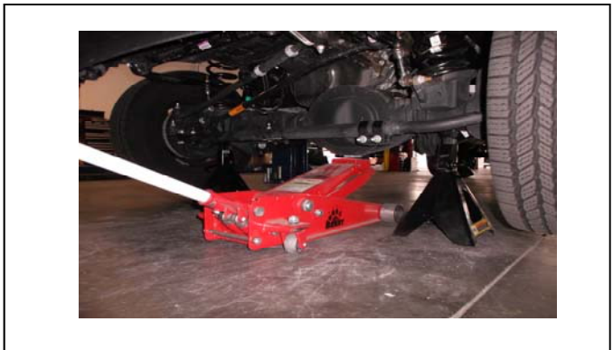
2. Lift the front of vehicle by the frame, then support the axle.
