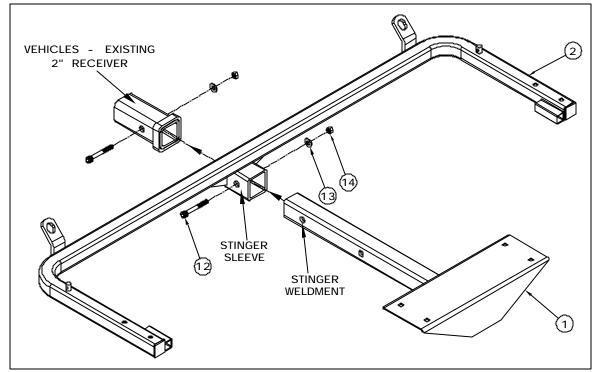
Insert stinger weldment into the stinger sleeve and tow vehicle's receiver to align 5/8" pin holes. Insert 7/16-14 x 2 3/4" cap screw (item 12) into receiver, tighten flat washer and 7/ 16-14 hex nut using the 11/16" socket and 3/8" allen wrench. Torque 7/16-14 hex nuts to 54 ft. lbs. Slide stinger sleeve back, align holes of stinger and sleeve. Insert 7/16-14 x 2 3/4" cap screw into hole, put on the 7/16" flat washer and 7/16 nylon hex locking nut. But do not tighten.
