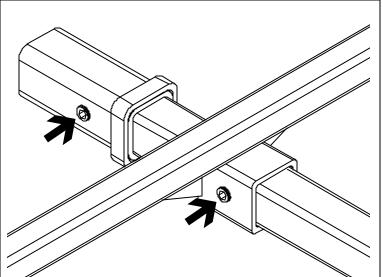
**NOTE:** The head of the 7/16-14 x 2 3/4" cap head screws are recessed into the 5/8" opening of receiver and stinger sleeve. This will allow stinger to be pulled to one side and eliminate stinger to wobble.
