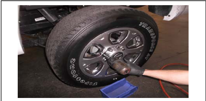
30. Reinstall the rear wheels.
