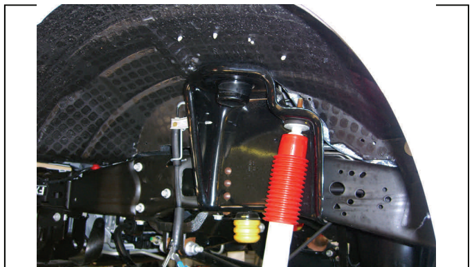
Carefully lower axle and remove coil spring
