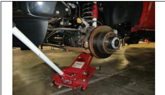
Support front axle with floor jack(s).
