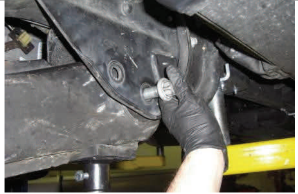
Support radius arm and remove attachment bolts
