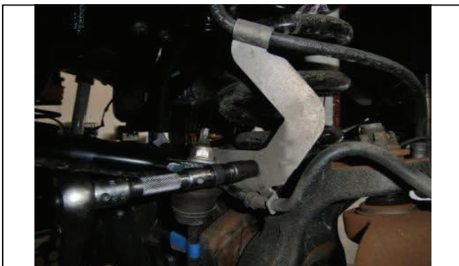
Disconnect brake line support bracket
